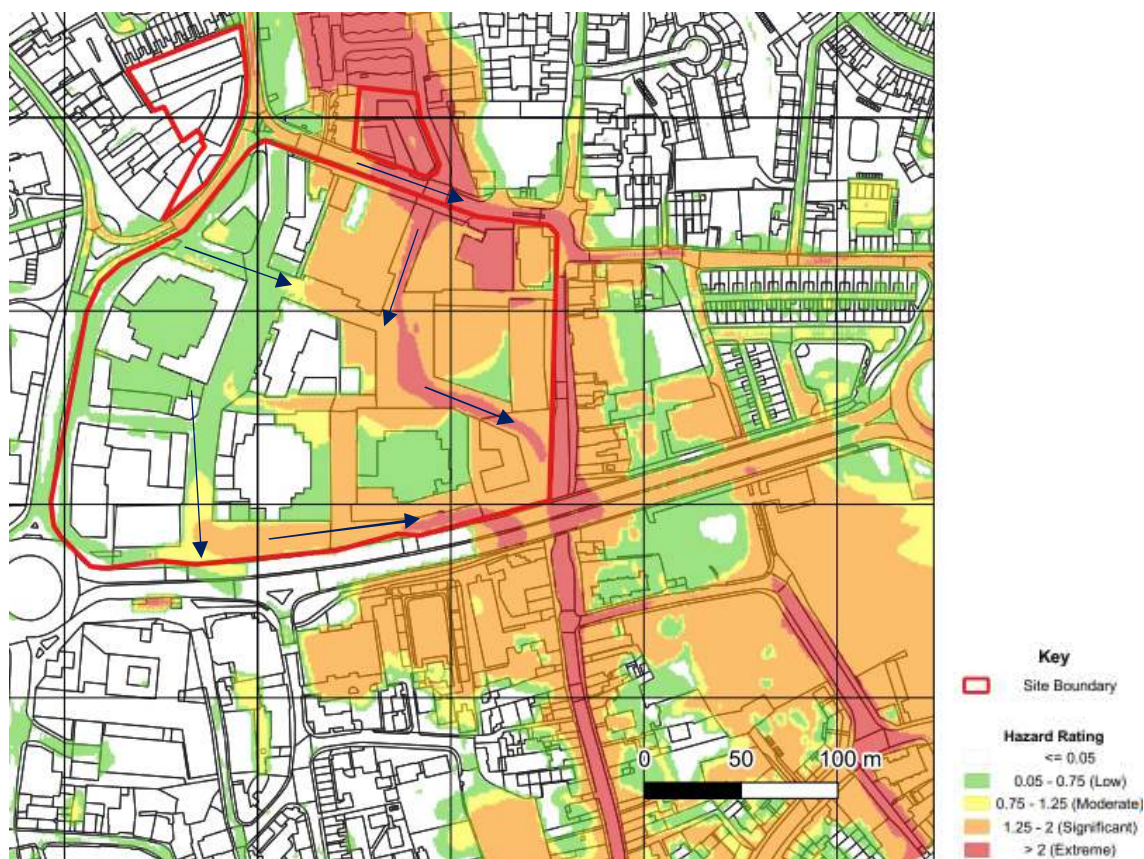
Figure 1: Velocity vector output for 1 in 100 year (+40%CC) surface water event – taken from Royal HaskoningDHV Report
