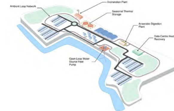
Fig 71 5G Ambient Loop Heat Network
